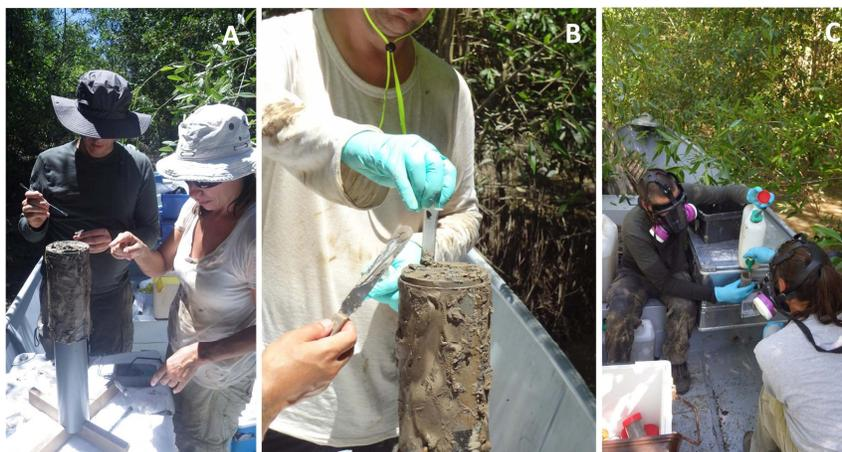
Figure 3. (A) Sampling of the sediment for the microbial analyses. (B) Sampling of the sediment for the analysis of the meiofauna. (C) Fixation with 4% buffered formaldehyde of the sediment samples for the benthic macrofauna and meiofauna analyses.
